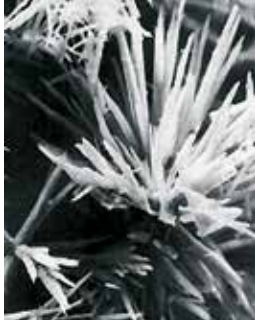
Picture 9: Lime protective layer
